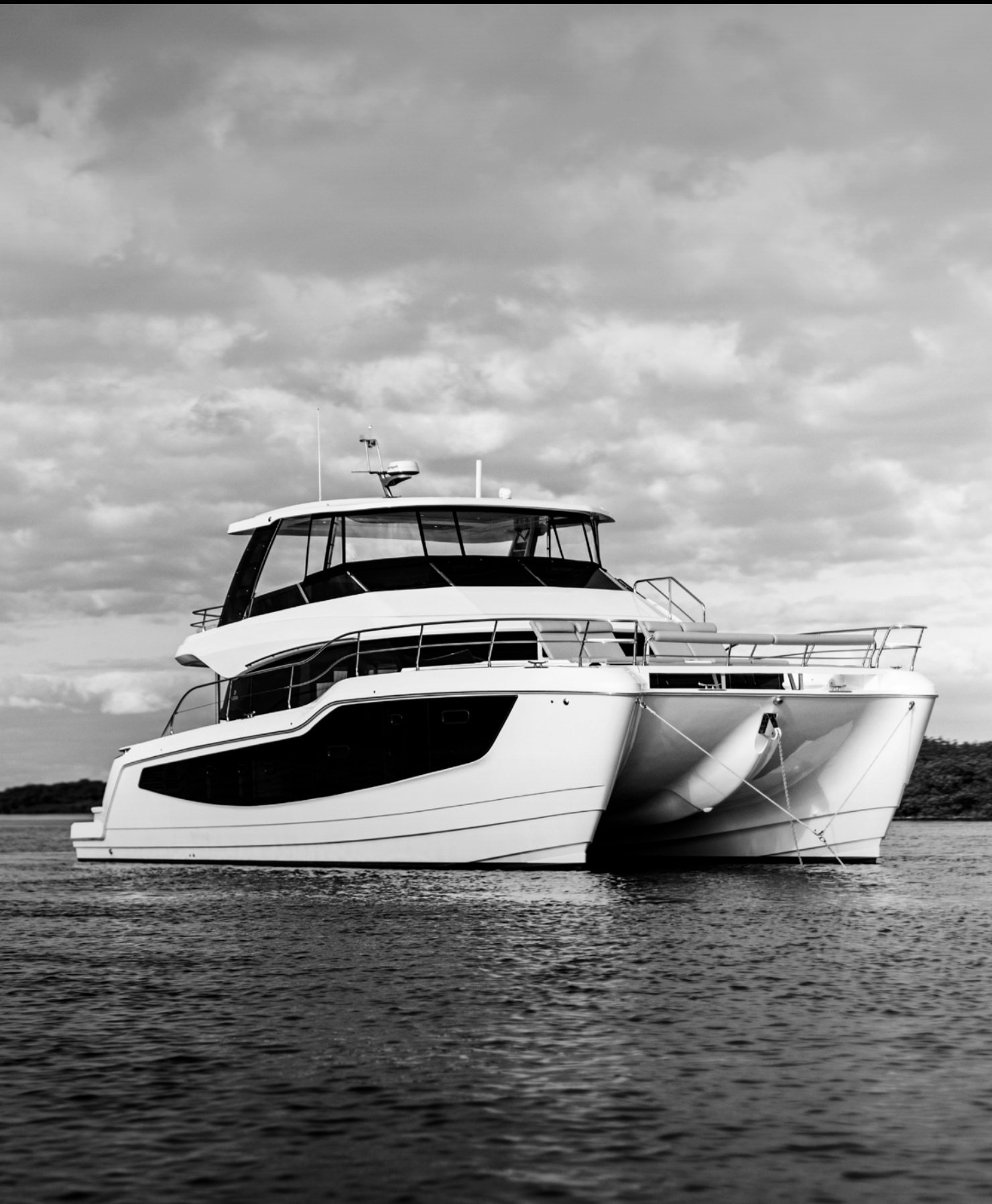
The Aquila 50's bow is designed to reduce spray generated when running into rough head seas.
